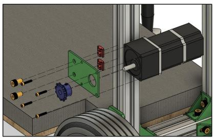
d. Fix wheel sprocket to drive wheel with bolt pattern, using <sup>3</sup>/<sub>8</sub>" by <sup>1</sup>/<sub>2</sub>" bolts [4] and <sup>3</sup>/<sub>8</sub>" nuts[4]
