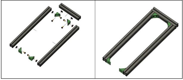
b. Connect upper frame assemblies to the lower frame, using corner brackets [8] and tee brackets [4] with M8 bolts [36] and T-nuts[36]
